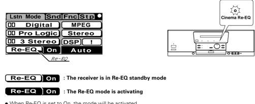
When Re-EQ is set to On, the mode will be activated automatically when in an effective surround mode.
